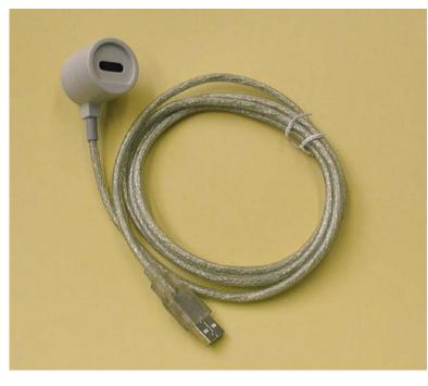
ANSI Type 2 Optical Probe with DTR Switch and USB connector for desk-top and lap-top computers.
