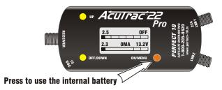
strength indicated on the bar graph(s) by minor azimuth, elevation and rotation adjustments of the dish. When you have maximized the readings, lock the dish mount bolts and re-attach the LNBfs to the switches or cables provided with the antenna. Then check your efforts with the satellite receiver.
