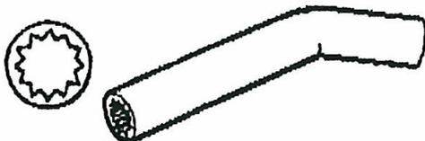
**Special Installation Tool for Vandal-Pruf Fasteners**
