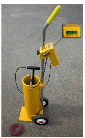
Pictured on the left is the 20 Kg version of the Clegg Impact Soil Tester. This model is designed for use on harder materials such as those employed in roadworks. Here the tester may be used in obtaining data for estimating the traffic carrying potential of lightly surfaced low traffic roads. Technical Note No 3 (Aug 97), available from SDi, reports the results of field tests
