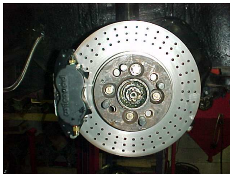
4 piston calipers with cross drilled and vented rotor
