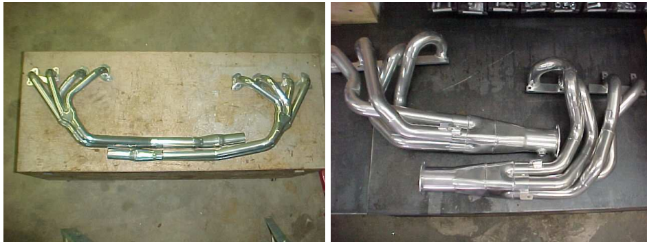
The 4 to 2 to 1 header (left) with a 1.5" diameter tubes and the 4 to 1 header (right) with a 1.75" diameter tubes designed by Lanocha Racing.
