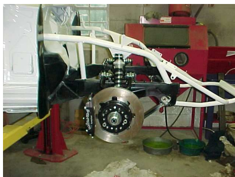
TR7 V8 with 6 piston calipers with a heavily modified front end and suspension
