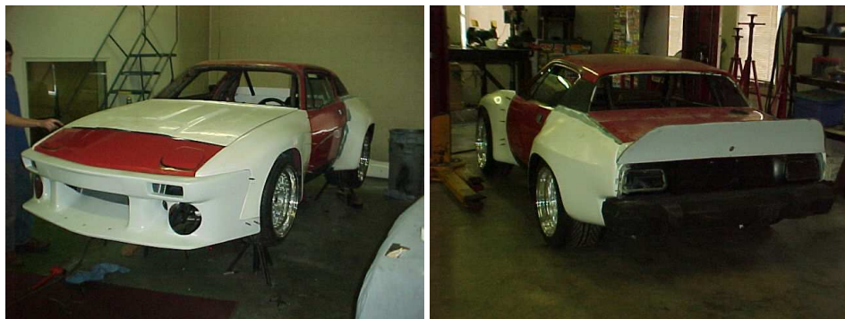
Body panels fitted and partially installed (left and right) including the rear spoiler (right) that bolts directly on.
