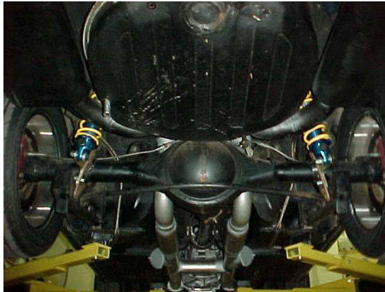
A Lanocha Racing TR8 with a Dodge/Plymouth 8-3/4 rear axle equipped with a coil over spring set-up and disc brakes. The coil springs were moved inboard to gain space for wider tires.
