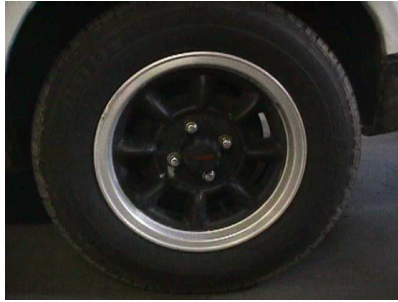
13-inch diameter magnesium rim
