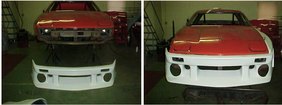
The front air dam was originally molded to be removable for transport. Clips and fasteners are needed for this panel
