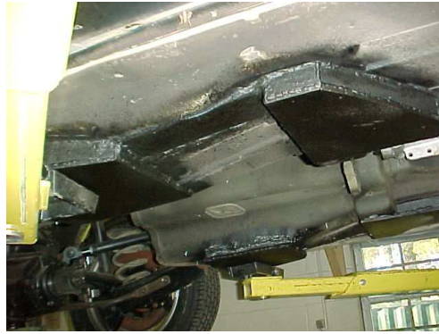
Finished with additional boxing of the rear arm mounting area and front frame member
