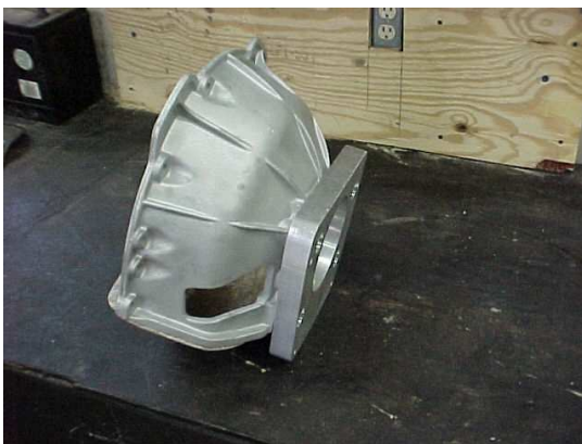
1961 to 1963 GM 215 bell housing for a T-10 with adaptor for a T-5 5 speed (left) and the adaptor for a T-56 6-speed on the (right)
