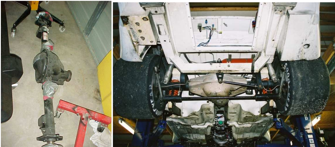
Ford 8.8 inch rear axle modified for the stock TR7/8 suspension arms (left) Group 44 Franklin Baby Grand rear axle (right)
