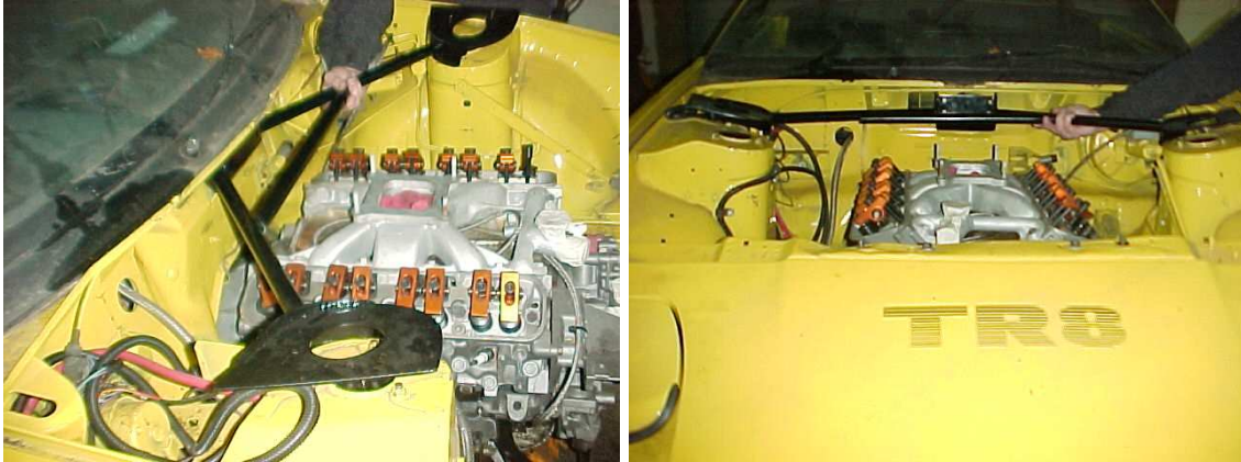
Strut brace being installed in to a TR7 V8 conversion car which is a bolt in item.
