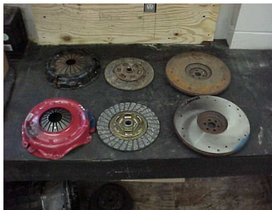
Stock TR8/Rover 3500 clutch assembly and flywheel (top) and the upgraded 10.5 inch diameter clutch disc, heavier pressure plate and a lightened flywheel a savings of 10lbs! (bottom)
