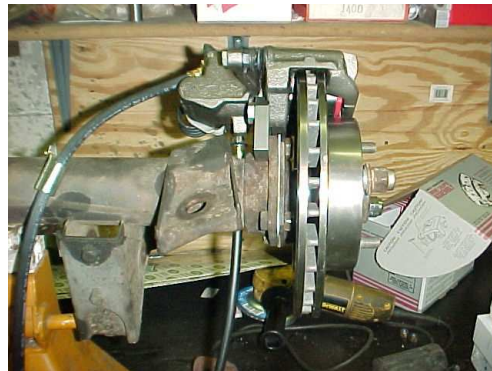
A work in progress for the stock TR7/8 rear end conversion to disc brakes (left and right)
