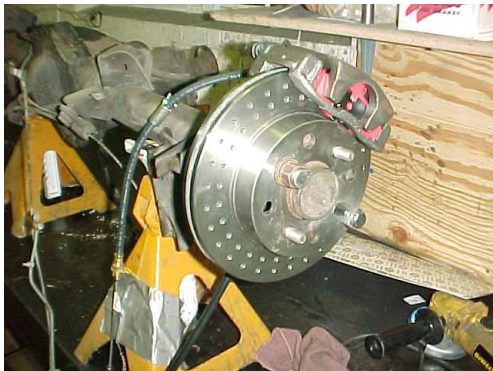
A work in progress for the stock TR7/8 rear end conversion to disc brakes (left and right)
