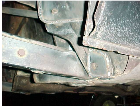
The upper and lower mounting points have been reinforcing with welded plates
