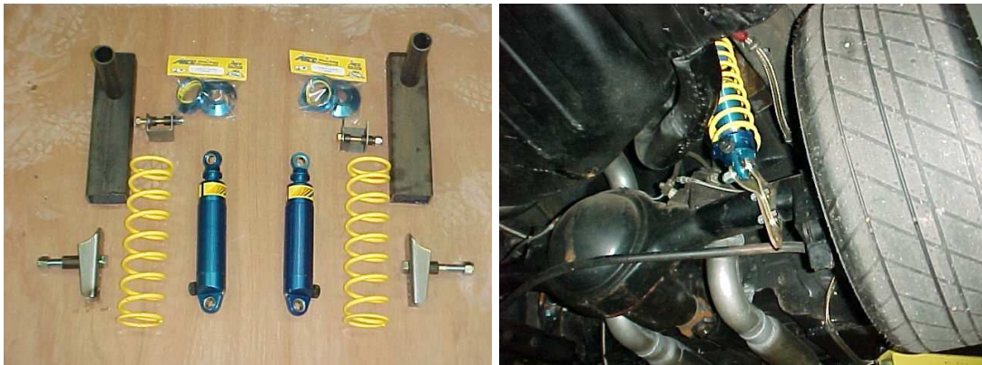
Coil over conversion kit (left) and the installed coil over assembly (right)
