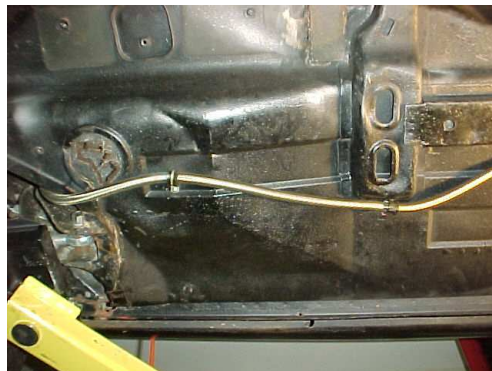
A typical torn floor pan that has reached the drain plug from the lower arm mounting point
