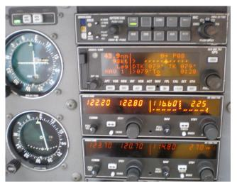
In this picture the Number 1 CDI NAV has been connected to the GPS signal. The NAV 1 VOR is set to 116.60 in the CDI mode and the OBS course is set to 225 TO. The aircraft is full scale (10°) to the right of the inbound course.
