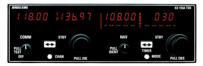
This NAV/COM has a lot of functionality. Like the audio panel much of it can be understood by expaned labels on each switch and display.
