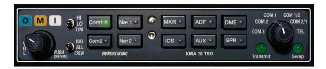
The **KMA 28** is pictured above. The model **26** is a slightly different, but understanding the operation of either model will enable you to operate the other without any difficulty.
