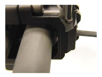
When contact is made, lock the screw in position with the 5/64 inch locking screw on the right side of the stock. The purpose of this screw is to control barrel whip during firing and is one of the things that enhances the accuracy of this system. If this step is not done correctly, the weapon will not achieve its maximum accuracy potential.
