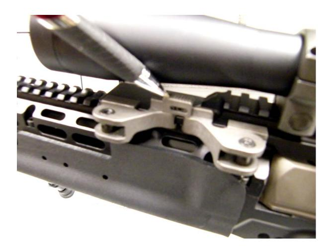
Once the lock has been disengaged, pull both levers out away from the base to unlock the base from the forward rail. This may require some force or the loosening of the screws on the throw levers using a 3mm allen head wrench.
