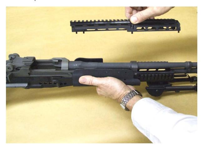
With the top cover / rail removed, turn the rifle over and remove the two 5/32 inch allen head screws that hold the forward hand guard to the lower rail.
