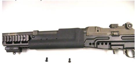
Re-install the top cover / rail assembly using the 6 5/32 inch allen head screws.
