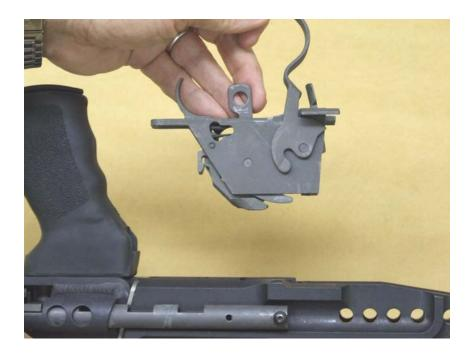
Reassembly is in the reverse order that this was accomplished and this is as far as the operator is authorized to disassemble the EBR. To prevent excessive wear of the stock components, this should not be done for cleaning purposes.
