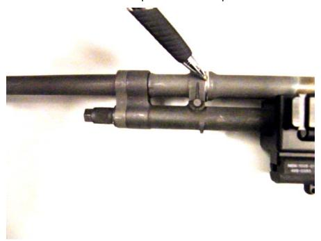
Verify that the Sage unique op rod guide is properly positioned on the barreled action. (Red dot should be facing the muzzle when installed correctly.) The Operating rod guide can only be installed one way.
