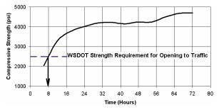
Figure 2. Compressive strength gain vs. time
