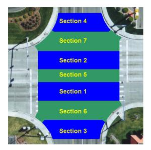
Figure 4. Concrete placement in interim Sections
