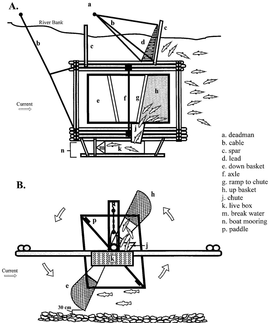
Figure 2.— Two-basket fish wheel used to capture chum salmon during the capture and recapture events; A: aerial view, B. side view.
