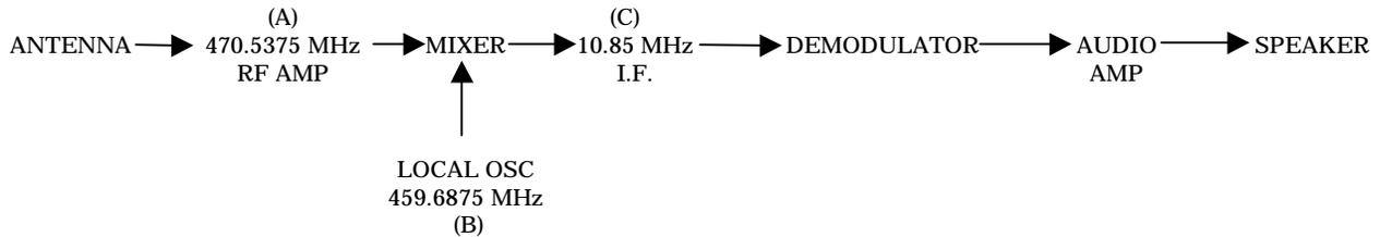
This receiver uses the same principal as the FM receiver we explored above except the local oscillator is now below the receiver frequency. This is called low side injection (the local oscillator is lower in frequency than the desired input frequency, Frequency "A"). Low or high side injection is a designer's choice. Either method will work equally well, and the superheterodyne process remains the same.
