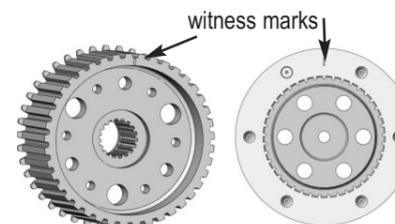
3. Align the witness marks on the pressure plate and inner clutch hub as shown when assembling.
