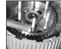
4. Check the Inner Stud Alignment using the clutch spring collar flipped over with the flange side in. The Collar should pass through the pressure plate freely a minimum of 1/4". Straightening is generally not required but if needed straighten the stud by using a small brass drift.
