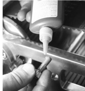
2. After all Pulley Caps are tight reinstall the outer support plate using Blue Loctite. Torque Bolt to 15-18ft lb.
