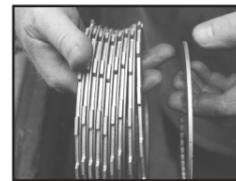
1. Ultima Belt Drive utilize the old style 900cc sportster steel drive plates and 9 special size fiber plates designed to provide a very adjustable Clutch Package. When Installing the Clutch Pack Install the Thick .119" Steel Plate First then Alternate Fiber/Steel. The Last Plate you install should be Fiber.
