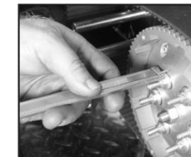
5. Install the clutch springs and clutch spring guides with the flanges out. Install the Clutch Spring nuts until you measure .350"+/- .010 from the face of the pressure plate to the face of the spring guide as shown. This sets the Spring at approx. 1.250 installed height. For higher power applications go in to .100" measured max for 1.000 installed height. Ultima Belt Drives come with a standard pressure spring for most applications under 100 hp.
