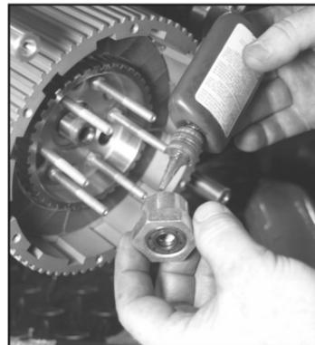
1. Install the clutch Basket Assembly onto the transmission mainshaft. Apply RED Loctite to the mainshaft nut and torque to 55-65 ft lb.
