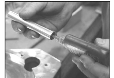
3. Using Red Loctite Install the remaining 5 long outer cover spacers with set screws into the Motor Plate. Motor Plates are drilled through so you can access the allen head from the inside. Put the Hex side of the set screw into the motor plate. Use Red Loctite on Outer Cover Spacers
