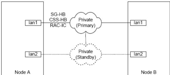
As illustrated in this picture, the primary and standby pair protects against single failure. Serviceguard monitors the network and performs local LAN failover if the primary fails. The local LAN failover is transparent to CSS-HB and RAC-IC. When both primary and standby fails, Serviceguard resolves the interconnect failure by performing a cluster reconfiguration. After Serviceguard completes its reconfiguration, SGeRAC notifies CSS and CSS updates RAC.
