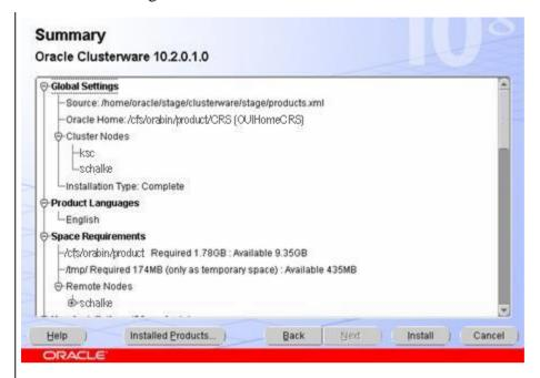
During the installation, the OUI first copies software to the local node and then copies the software to the remote nodes.
