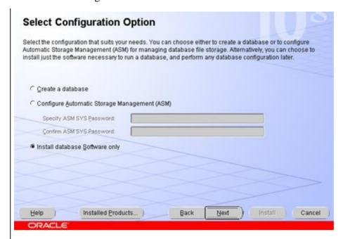
Here we recommend only to the software and not to create a starter database. We will create a database later with the Database Configuration Assistant.
