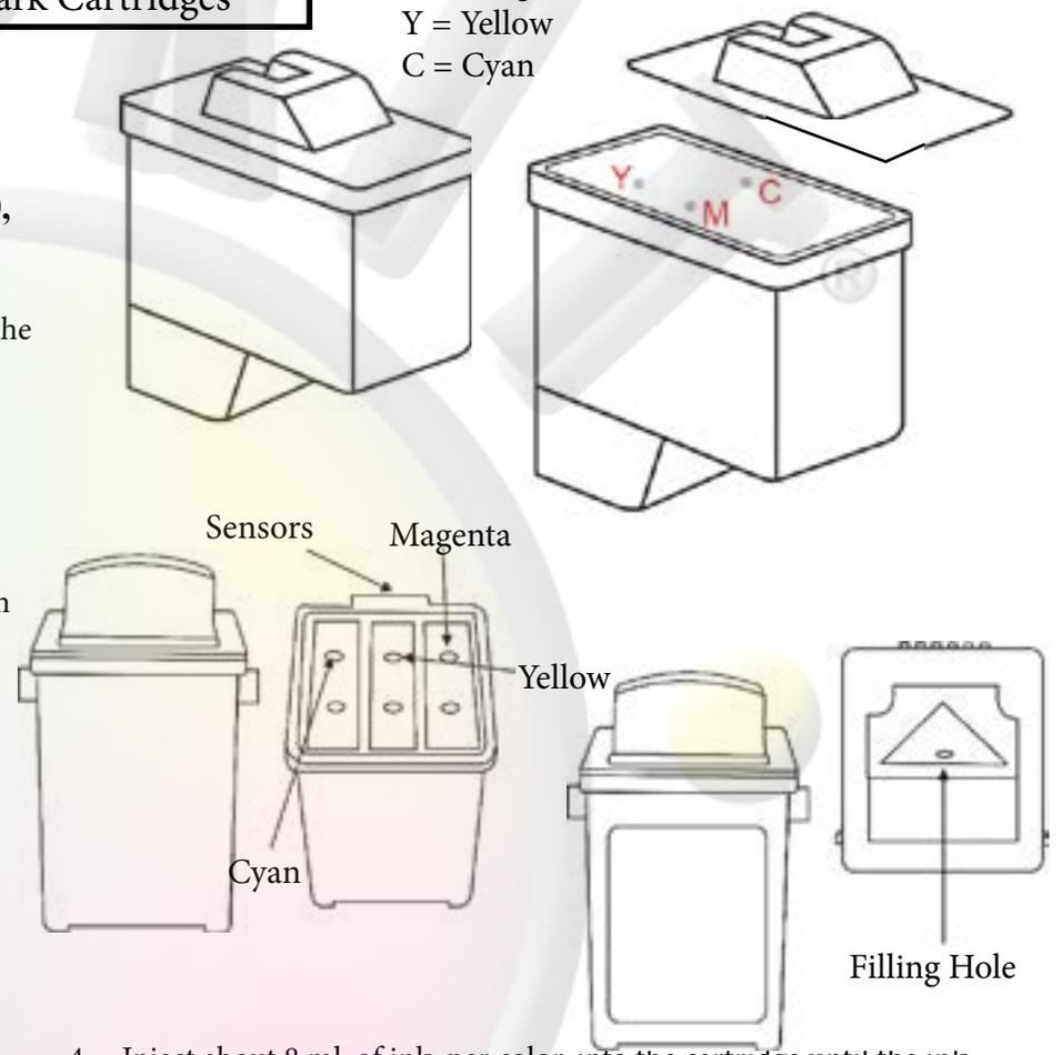
4. Inject about 8 ml. of ink, per color, into the cartridge until the ink begins to bubble at the top of the sponge. Important: Do not overfill. Keep the sponge inside the cartridge white.
