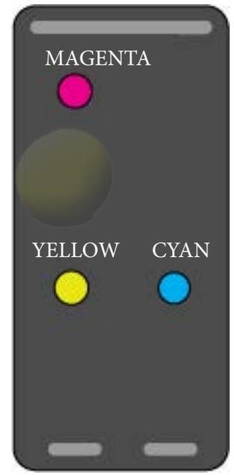
**NOTE:** *If your cartridge is part of Lexmark's recycle program, then the refilling holes might not be viewable. In this case you can drill a hole in the same area's indicated above to refill the cartridge.*
