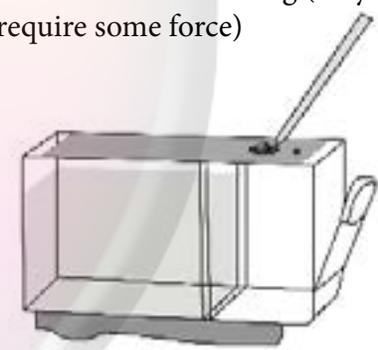
Method 2. If you feel that the first method of refilling is not something you'd like to try, you can place ink into the cartridge via the nozzle. By turning the cartridge over so that the nozzle (Outlet Port) points up, you can slowly drip ink into the nozzle. This procedure may take long and no ink will go into the ink chamber, but the sponge will retain some ink for you to use and continue the use of your cartridge. You may usually use about 3-4 ml of ink at a time in the sponge.
