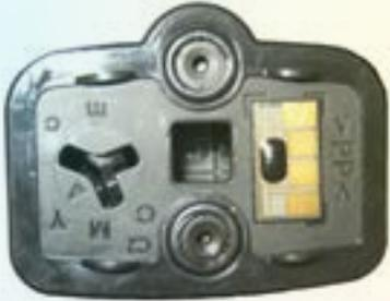
The illustration above is the bottom part of the cartridge. The chip is located on the right side in this example. To remove it, you will need a small flat head screwdriver. When ready, pry the chip from the cartridge.
